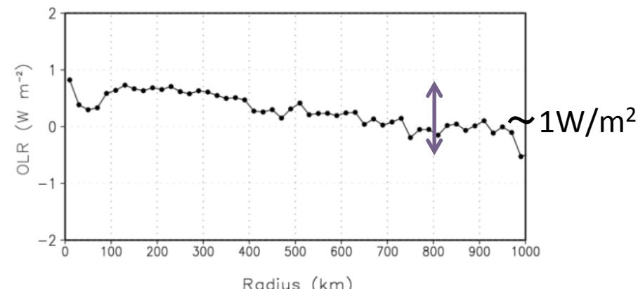
It maybe difficult to discuss a budget for  $r < \text{ca. } 80\text{km}$  because the net error in  $\Delta F$  (i.e., sum of the errors of present + future) is larger in a smaller radius range ( $1.7\text{W/m}^2$   $r \sim 80\text{km}$ )
