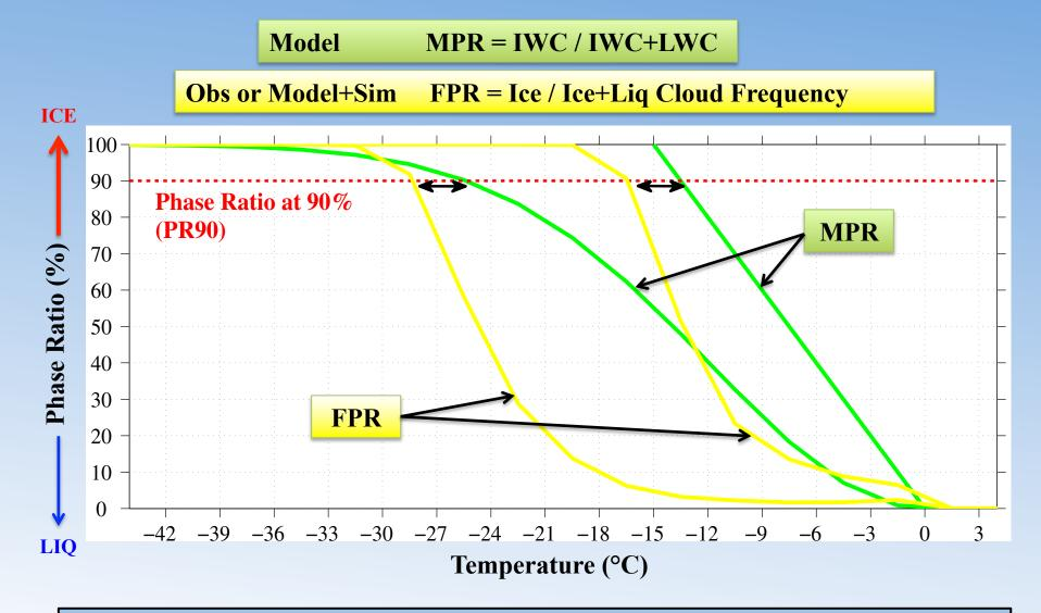
At 90%, Mass Phase Ratio (Model) ≈ Frequency Phase Ratio (Obs) → PR90 allows a consistent evaluation of the models <u>while no simulator is used</u>.
